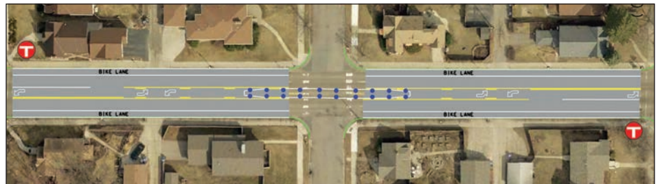
East 46th Street at Oakland Avenue. Enhanced pedestrian crossing is indicated by blue dots.
